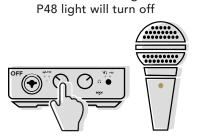
Set input level with left knob while checking signal light
