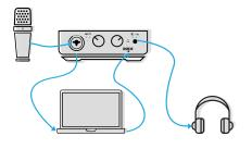
If using powered speakers, disconnect headphones to activate the balanced speaker outputs
